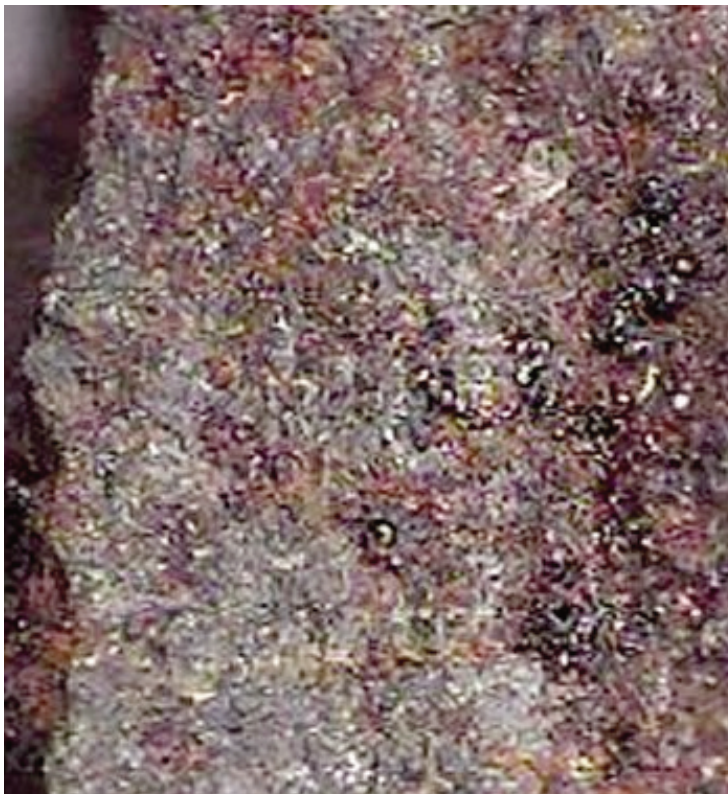
Specimen of volcanic rock containing dark grey grains of native iron (pictured above) This locality is one of the very few known localities for terrestrial native iron. Location : Disko Island, Greenland
